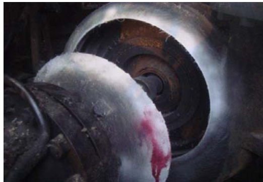
Casing plate of crude booster cut circumferentially by rubbing action of impeller.
