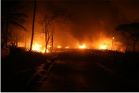
A loaded LPG Bulk TT, on its way to the unloading destination, was travelling on National Highway when it was involved in an accident at a major intersection. Consequently, there was LPG leakage, vapor cloud formation, fire and, finally, BLEVE causing devastation – loss of more than 20 lives and extensive damage to property of the population living nearby.
